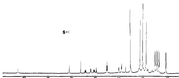
Figure 3. The proton NMR spectrum of 3-iodorifamycin S in chloroform- d at 270 MHz.
